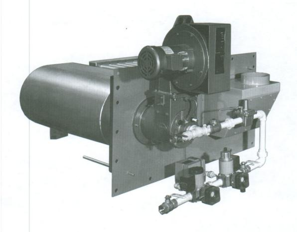
Eclipse Recirculating Low Temperature (RLT) and Recirculating High Temperature (RHT) indirect air heating burners are designed to heat recirculating ovens and dryers where the products of combustion must be isolated from the process air stream. They are also excellent for use in industrial space heating systems. These burners feature an industry-proven burner, firing chamber and exhaust tubes assembled as a single unit for easy installation and optimum performance.
